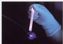
SON - Arc Tube Test by Tesla Coil (7)
