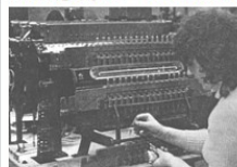
Emitter Coating of SOX Cathodes (8)
